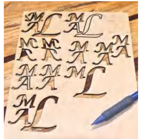
▲ Pic.18 The letters were cut out of 1.5mm maple plywood by a local company that uses a laser. The cost was minimal for the laser cutting and cutting the 1.5mm deep holes in the lid to match the inlaid monogrammed initials. I have absolutely no talent for free hand carving!
